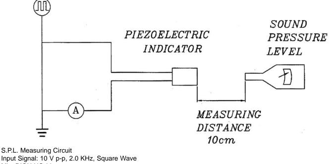
Input Signal: 10 V p-p, 2.0 KHz, Square Wave Mic: RION UC 30 S.G.: Hewlett Packard 33120A Function Generator or equivalent
